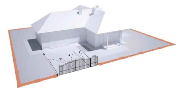
Before commencing installation it is necessary to determine the place of fencing installation. The area should be properly prepared and organised. Next, it is necessary to establish the direction of gate and wicket opening and take into account the dimensions of fencing constituents and distance from buildings.
