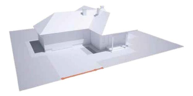
After establishing the location and taking all the dimensions into account, it is possible to commence making excavations for the purposes of strip footing, and preparing the reinforcement. (see pages 10 and 11)
